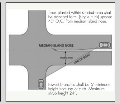
older, typical design method. I am working through the process of incorporating the Chico design standards into the design standards for future median islands here in Hayden.
