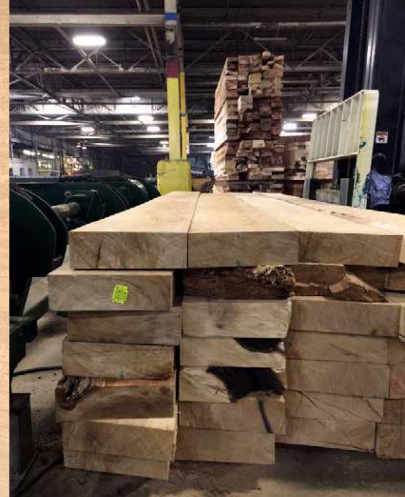
Upcycled urban timber at Sterling Lumber milling facility in Phoenix, Illinois. Logs produced from municipal/public property ash removals were milled and used in the shipping and construction matting industries. Photo by Jim Semelka
